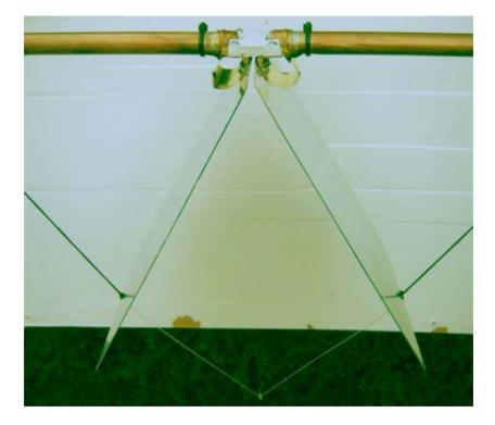
Here's another view of the loop with the tuning plates and elastic cords fitted
