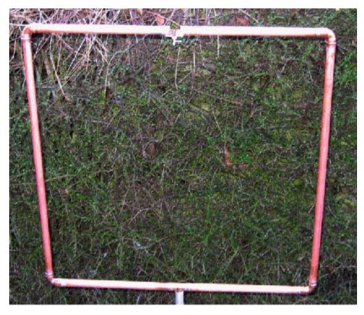
I decided to mount the brass hinges by cutting a slot in the end of the pipe and soldering them directly in.
