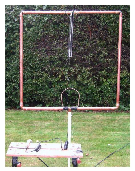
The tuning range of the loop with this size of plate was approximately 9MHz to 25MHz.
