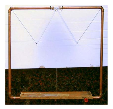
This is the loop under test on 10MHz; note the relative size of the coupling loop. The small size indicates that the loop has low losses resulting in a 'high 'Q' factor.
