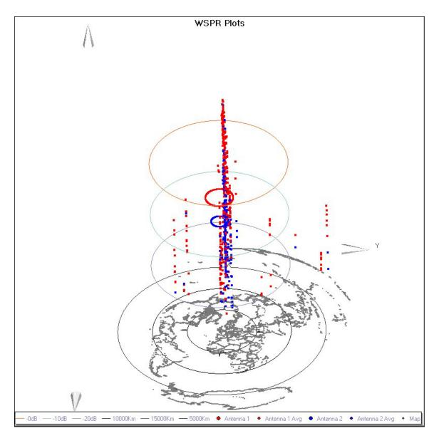
The red trace is obtained using the 30m doublet and the blue traces using the 1m loop.
