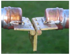
The next stage is to fit the tuning plates on to the hinges and make a Perspex plate to mount across the top faces of the hinges to hold them apart at the correct spacing. I may also have to use a spacer between the tops of the hinged plates to stop them shorting as they swing open. Some short straps made from thin brass sheet connect between the two halves of the hinges in order to ensure a good low impedance moving joint.
